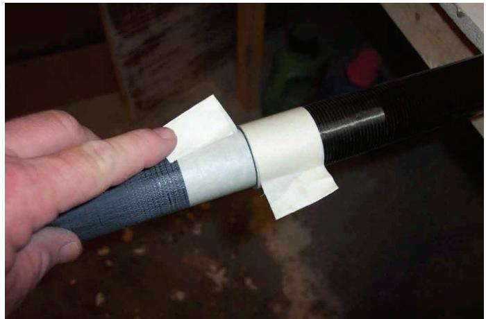
Decide where you will be doing the first part of the fabrication and move all the parts to this area. Mix about 2 tbs of JB Weld on a clean surface and follow the Mfg. instructions. When mixed, move this close to the work area. Remember...protection, this stuff gets everywhere.
