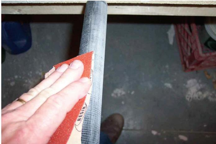
. Next, hand sand the outside of the ferrules. This should be a 98% sand meaning the entire surface needs to be sanded. You can use the "shoe shine method" or length-wise, either is fine but do not over sand. Once the surface is abraded that's when you stop. Clean with a dry clean cloth. There should not be any dust left on the surface.
