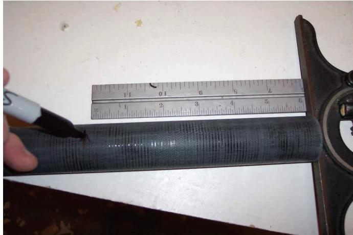
I found it easier to flatten the point of the tip to the diameter of the head of the #14 screw first before I began drilling. This gave me a flat surface to begin drilling. You can flatten the point using a bench grinder, disc sander or just a piece of coarse sandpaper placed on a flat surface and move the tip against that.
