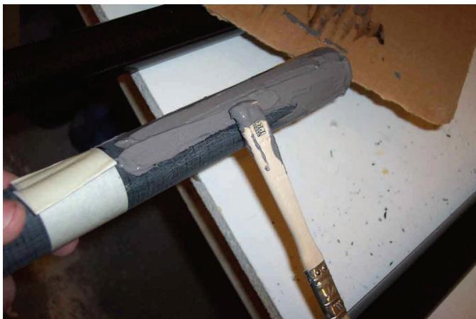
Set that down and butter the ferrule..use a bit more on the ferrule than inside the tubing.
