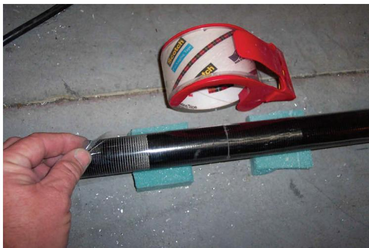
Now take about a 12" piece of the 2" cellophane mailing tape and use it to tape the section(s) lengthways..this will keep the section from moving a great deal while you are working on the next one. Last, install the point.
