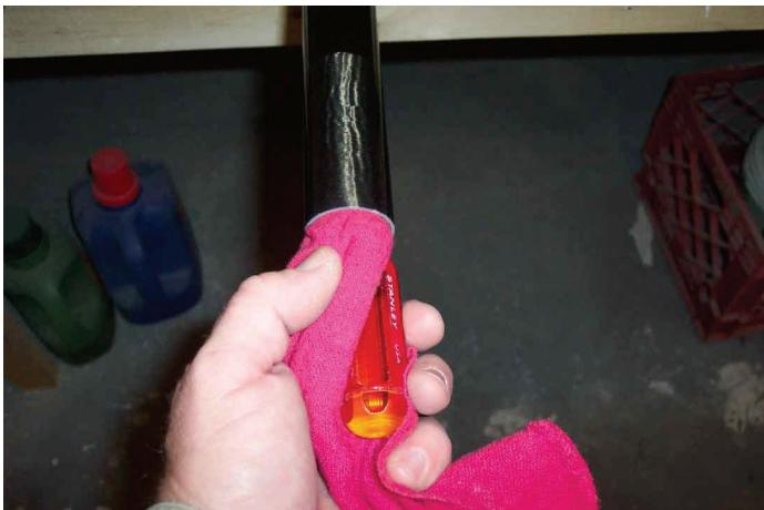
Step one: First wipe the inside of the pole tubes with (and I'll just use this from now on to make it simple to write...you have a few choices for solvents) acetone. Use a clean rag and make sure you get at least 6" to 8" inches wiped. Wipe the outside of the ferrules. This will remove all of the mold release on these parts.
